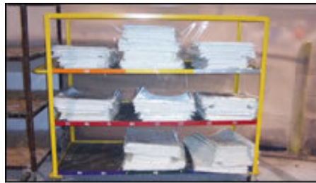
Fiberglass Rack reconfigured & sequence-stacked for laying up a boat hull
