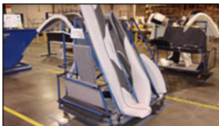
Pull System Project - Using a limited number of racks for upholstery kits.
